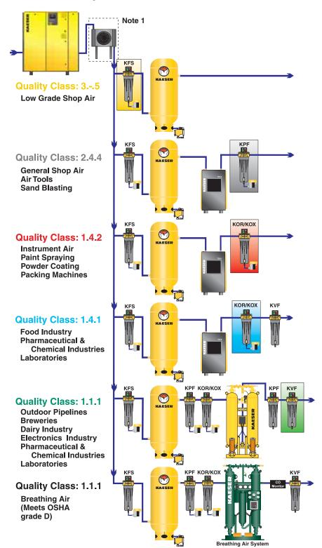
Note 1: All Kaeser Rotary Screw Compressors have built-in aftercoolers. However, for equipment without an aftercooler or where the discharge temperature is 110°F or higher, an aftercooler should be positioned at the location shown.
